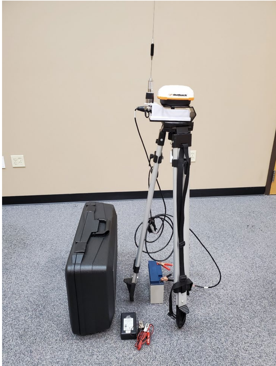
Figure 1-1: Outback Guidance A631 RTK Base Station
