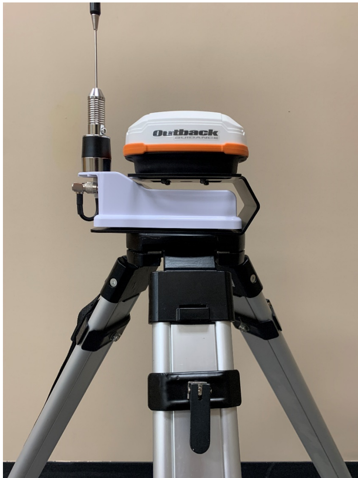
Figure 2-2: A631 RTK Base Station on Tripod
