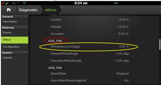
If the voltage ranges are outside of the Min/Max, you will need to adjust the WAS. So far, we have seen few cases where the WAS itself needs replaced due to malfunction. As always, check your cables, pins, connections, and swing arm movement when troubleshooting the WAS.
