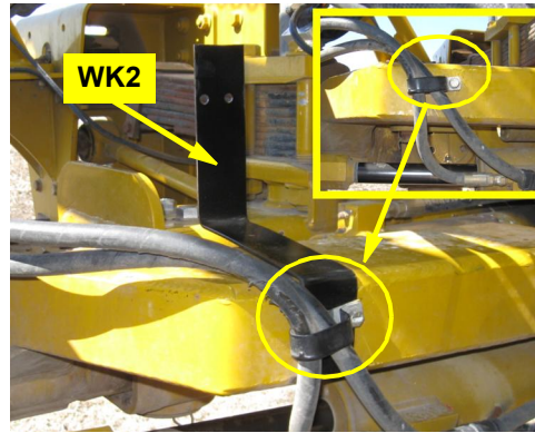
Figure 2a with inset: Installed WAS mounting bracket
