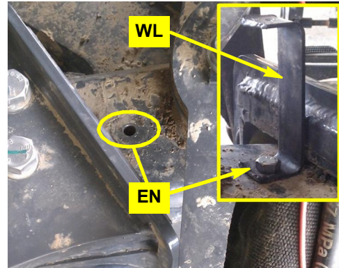
Figure 2b with inset: WAS link rod mounting bracket installed
