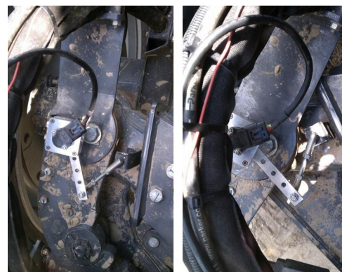
Figure 2e: Full left lock (left image) and full right lock (right image)
