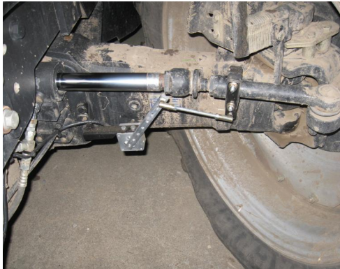
Figure 2f-i: Installed WAS - full left lock
