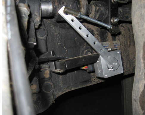
Figure 2e-ii: Installed WAS - full right lock
