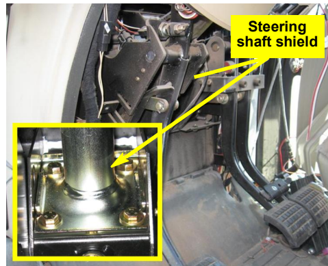
Figure 1b with inset: Console panel removed. Steering shaft shield between pedal mounts
