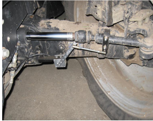
Figure 2e-i: Installed WAS - full left lock
