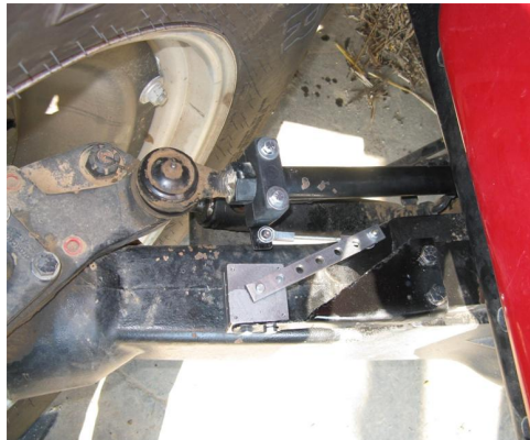
Figure 2f-i: WAS at full right lock
