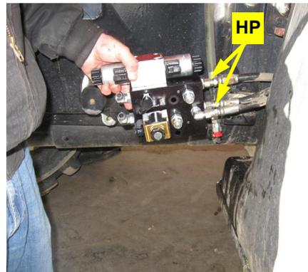
Figure 4b: Steering output hoses connected to the hydraulic block
