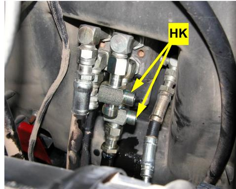
Figure 3b: Installed run-tee fittings and re-connected steel line fitting
