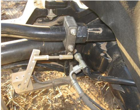
Figure 2f-i: Installed WAS - full left lock
