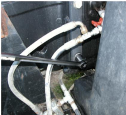
Figure 2a: Removing lower step mounting bracket bolt
