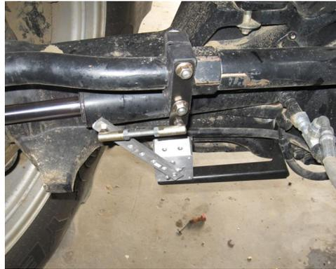
Figure 2f-ii: Installed WAS - full right lock
