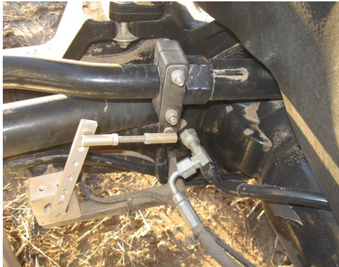
Figure 2f-i: Installed WAS - full left lock
