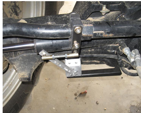
Figure 2f-ii: Installed WAS - full right lock
