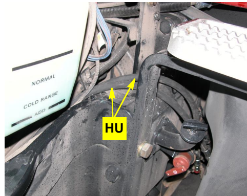
Figure 2b-ii: Routing the steering output hoses—following the machine's steering lines
