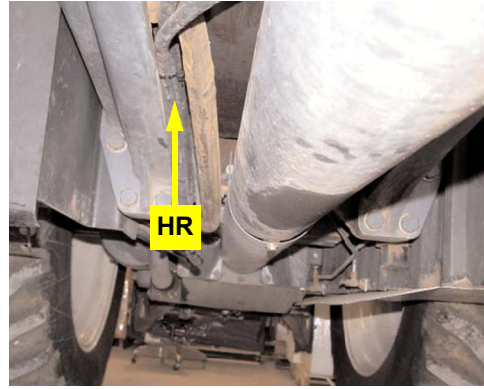
Figure 5c-i: Steering hoses routed to steering block
