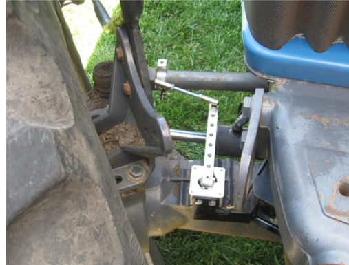
Figure 2f-i: Installed WAS - full left lock
