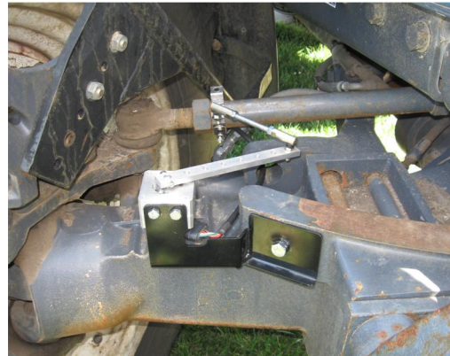
Figure 2f-ii: Installed WAS - full right lock
