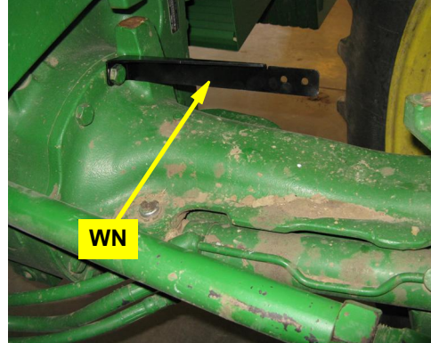
Figure 2a-ii: Installed WAS mounting bracket
