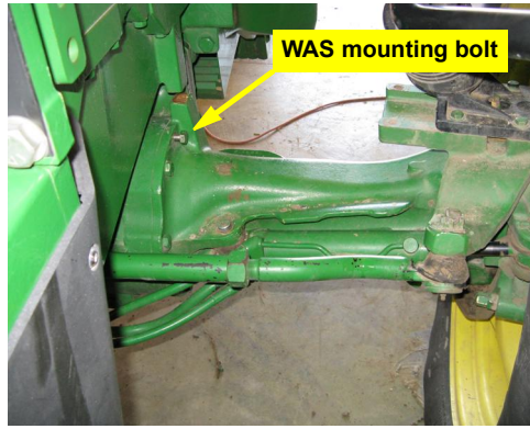
Figure 2a-i: WAS mounting bracket location
