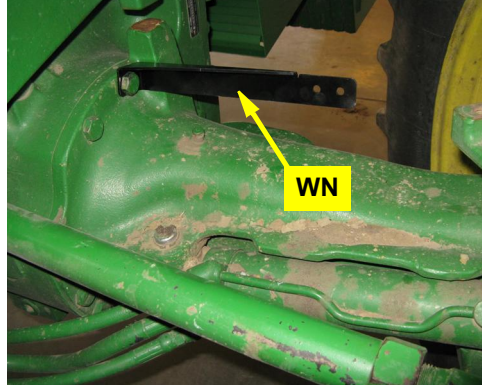
Figure 2a-ii: Installed WAS mounting bracket
