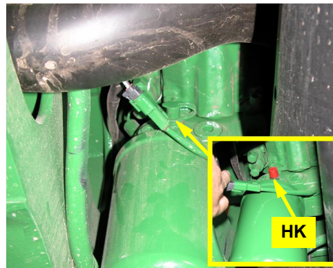
Figure 5b with inset: Installed tank fitting
