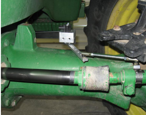
Figure 2e-i: WAS at full left lock
