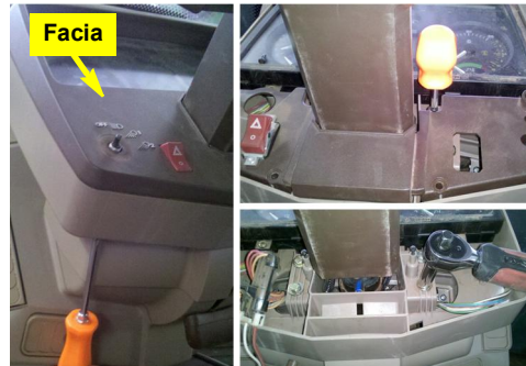
Figure 1a: Dismantling the upper console set
