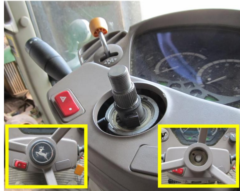
Figure 2a: Steering wheel removed
