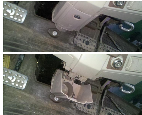
Figure 4a: Releasing the front section of lower console set
