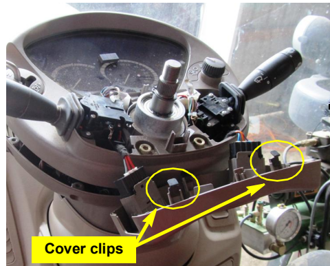
Figure 2b: Switch box cover removed
