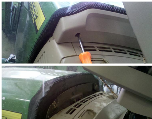
Figure 4b: Removing forward, top section of lower console set (top image) and section removed (bottom image).
