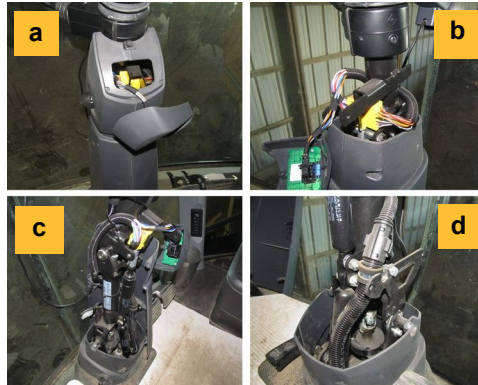
Figure 2 a-d: Dismantling the console
