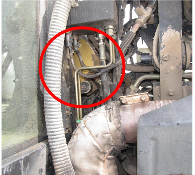
Locate the enable solenoid on the side of the block. Plug in the 2 pin connector from the 051-0466-10 harness into the enable solenoid.
