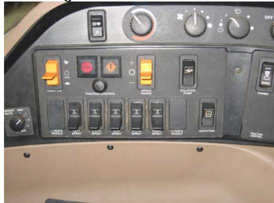
Fig. 8: Boom Sections Off
