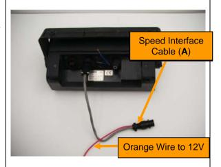
4. Connect the opposite end of the Speed Interface Cable to the S-Lite power cable.
