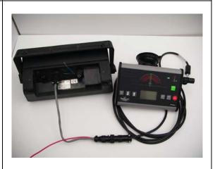
5. Be sure the controller is collecting data from your speed interface cable by driving the tractor and watching the controller.
