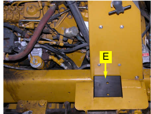
Figure 2b. Installed mounting bracket.
