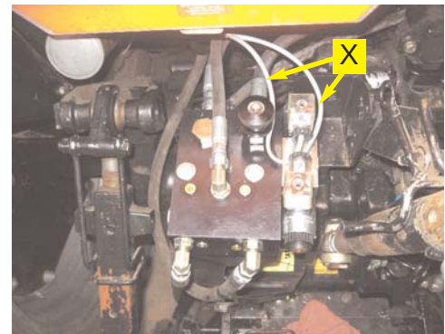
Figure 8a. Installed valve cable at the automated steering block.
