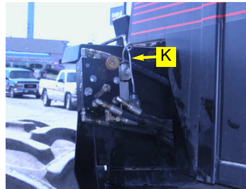
Figure 7a. Installed valve control cable.
