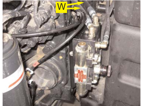
Figure 8b. Installed steering lines..
