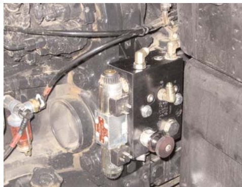
Figure 2c. Mounted automated steering block.
