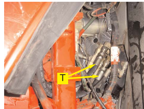
Figure 5a. Steering hoses at the orbital.
