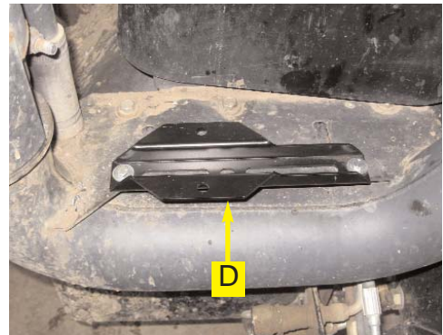
Figure 2b. Installed mounting bracket.
