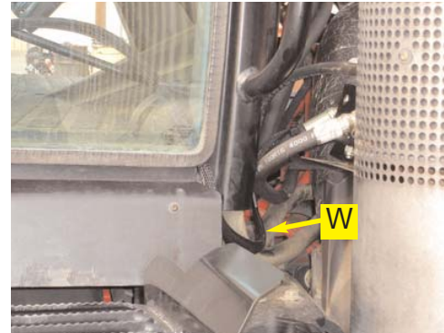
Figure 10b. Valve cable routed into the cab.
