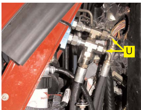
Figure 5d. Steering hoses at the counter-balance valve.
