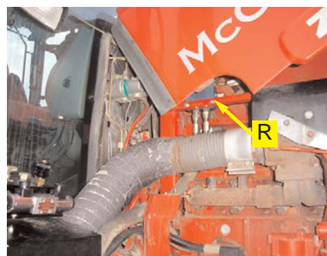
Figure 4b. Installed counter-balance valve block.
