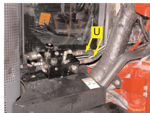
Figure 5c. Steering hoses at the automated steering block.
