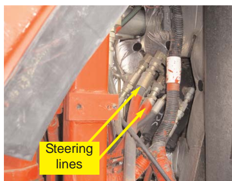
Figure 4c. Steering lines at the steering orbital.
