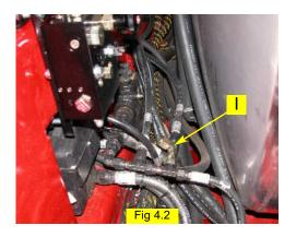
Locate the steering orbital under the sprayer cab (Figure 4.3) and install the run-tee (I) into the return line at the steering orbital as shown. (Figure 4.4) This will provide a tank return for the hydraulic control block. Use plastic caps to prevent excess leakage from the run-tees during installation.
