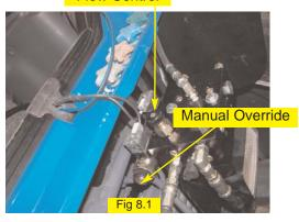
**Note:** To activate the manual overrides, a tool such as a small screw driver or allen wrench must be inserted into the end of the coil to depress the override button.
