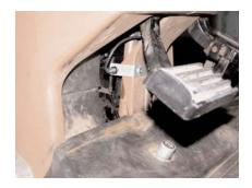
**Connect to Console:** Connect the magnetic sensor to the automated steering console accessory port using the provided interface cable. Secure the sensor cable and interface cable with tie straps and route as desired.
