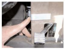
**Install Magnets:** Clean the steering shaft thoroughly where the magnets will be installed. Mix equal amounts of the 2-part epoxy provided. Apply epoxy mixture to one side of each magnet and install the magnets vertically on to the steering shaft 180 degrees apart. Let the epoxy cure for 5 minutes.
