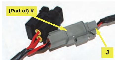
Figure 5c: Power cable to junction box cable
