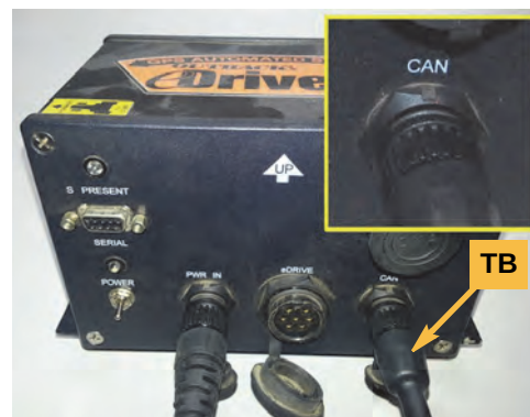
Figure 1c with inset: CAN cable connection at ECU
