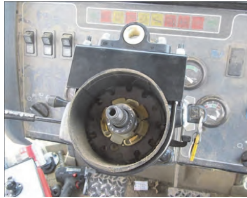
Figure 5: Anti-rotation assembly installed
