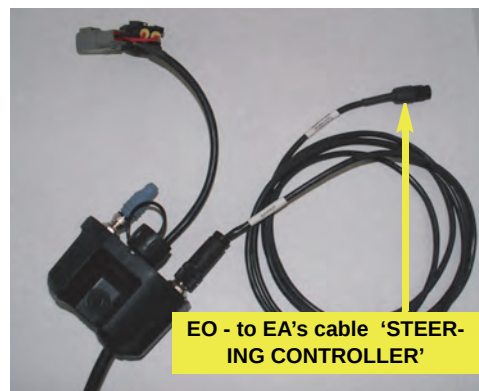
Figure 7e-ii: CAN cable to eDriveX
