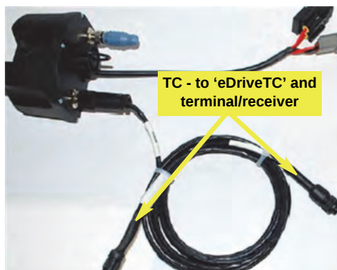
Figure 7e-i: CAN cables to eDriveTC and terminal/receiver
