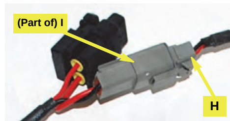
Figure 5c: Power cable to junction box cable
