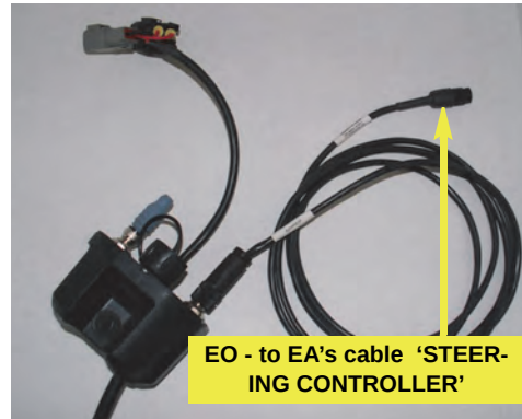
Figure 5e-ii: CAN cable to eDriveX
