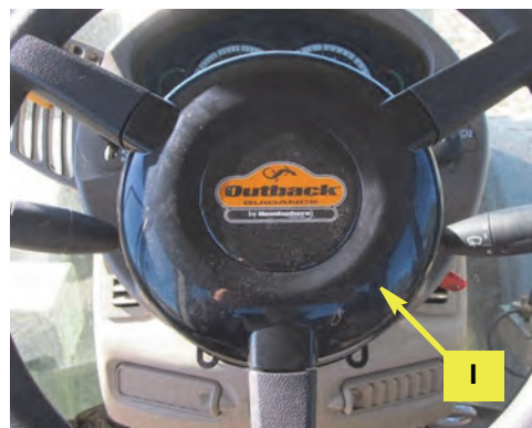
Figure 4b: Steering wheel center cover installed
