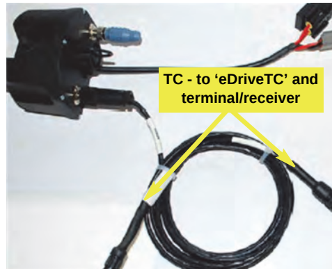
Figure 5e-i: CAN cables to eDriveTC and terminal/receiver
