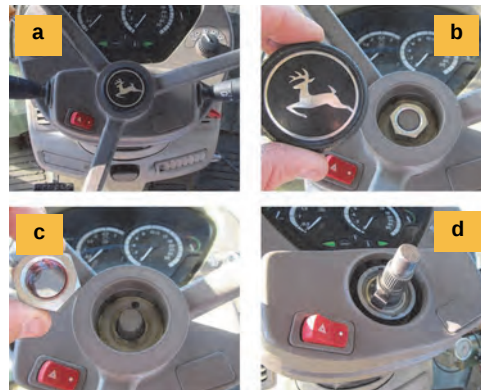
Figure 3 (a-d): Removing the steering wheel
