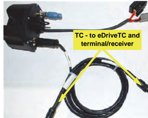
Figure 5e-i: CAN cables to eDriveTC and terminal/receiver
