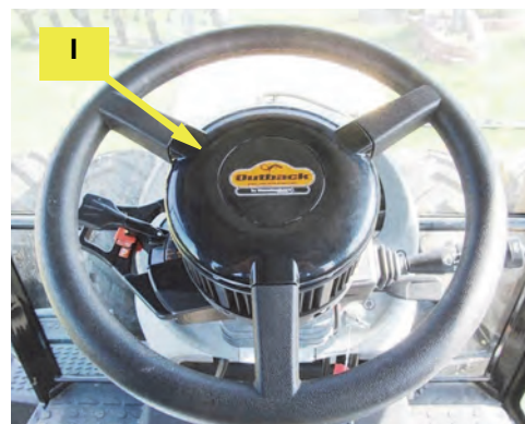
Figure 4c: Center cover installed
