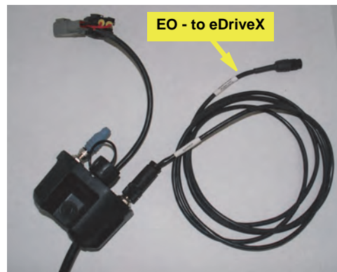
Figure 5e-ii: CAN cable to eDriveX
