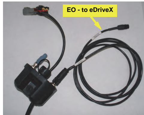
Figure 5e-ii: CAN cable to eDriveX
