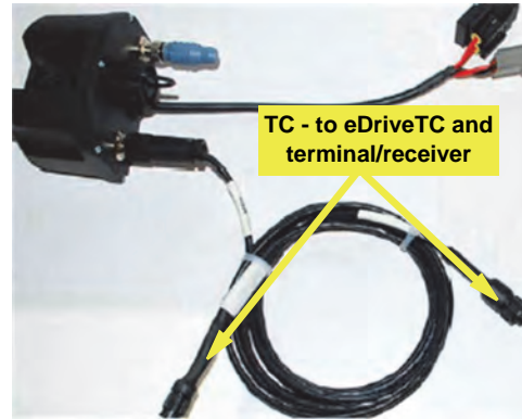
Figure 5e-i: CAN cables to eDriveTC and terminal/receiver
