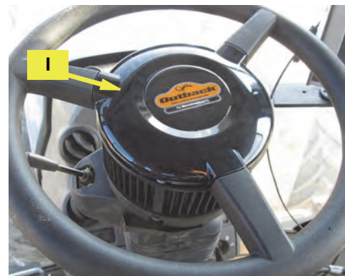
Figure 4c: Center cover installed
