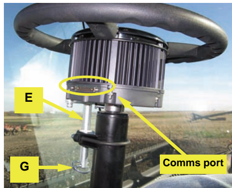
Figure 5a: Steering assembly mounted on steering shaft. Linchpin installed.
