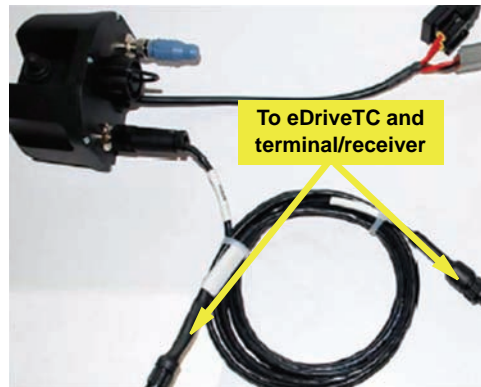
Figure 6e: CAN cables to eDriveTC and terminal/receiver
