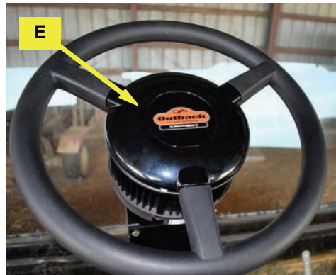
Figure 3c: Installed center cap
