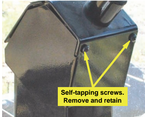
Figure 3e-ii: Plain metal steering column screws
