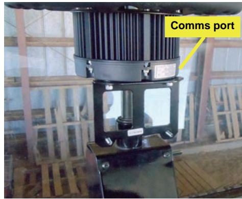
Figure 3a: Installed steering wheel assembly
