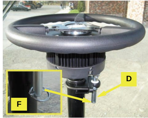
Figure 5a with inset: Steering wheel assembly and linchpin (inset) installed
