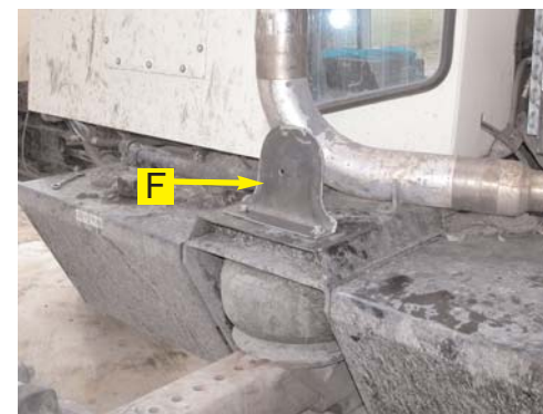
Figure 2b. Installed mounting bracket.
