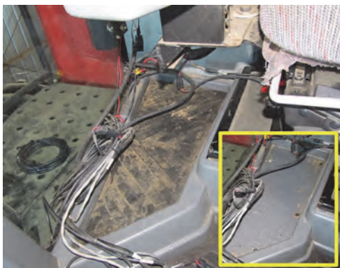
Figure 2f with inset: Accessing the cab access hole
