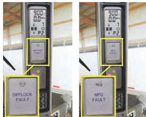
Figure 2c: Wrong WAS adapter cable warnings
