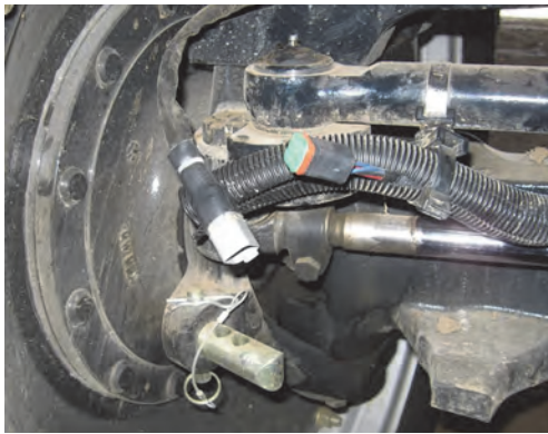
Figure 2d-ii: Disconnected 6-pin connector
