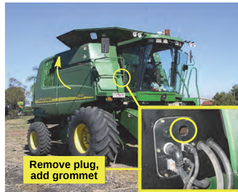
Figure 3b-i with inset: Opening a cab access hole - STS
