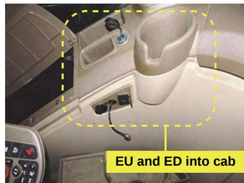
Figure 3c-ii: Cabling in/out of cab access area - S-Series
