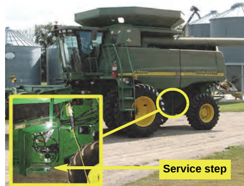
Figure 1a with inset: Compartment (inset) and compartment location
