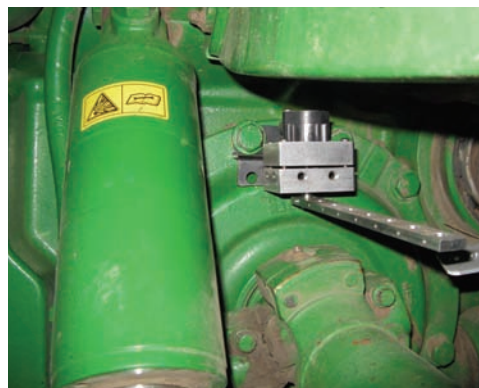
Figure 2c: Installed WAS assembly
