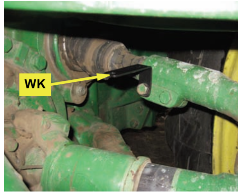
Figure 2d: Installed WAS rod mount
