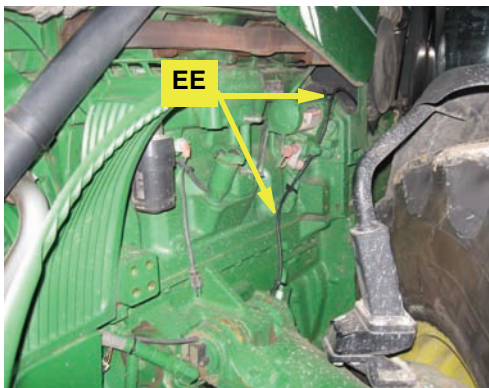
Figure 2c-i: WAS cable routing cab to front axle
