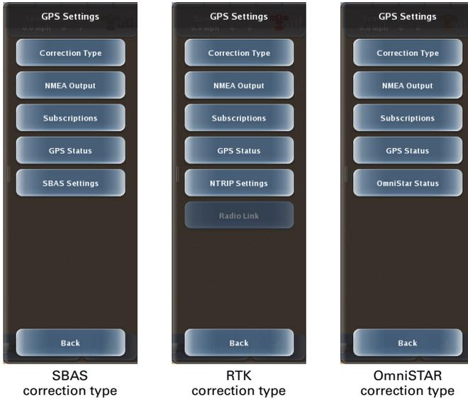
**Figure 1-6: Correction types and related GPS Settings panel buttons**
