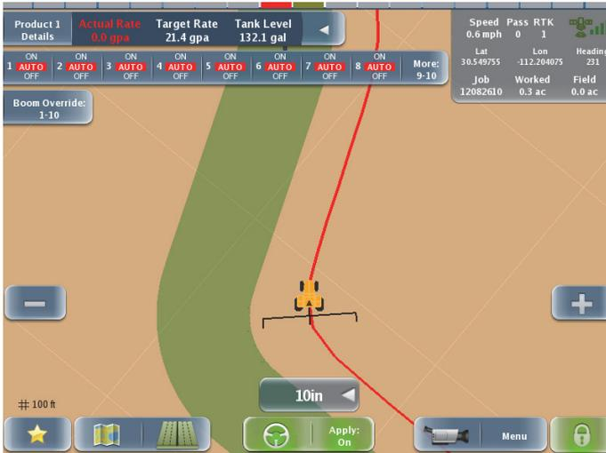
**Figure 6-3: Contour Lock mode**
