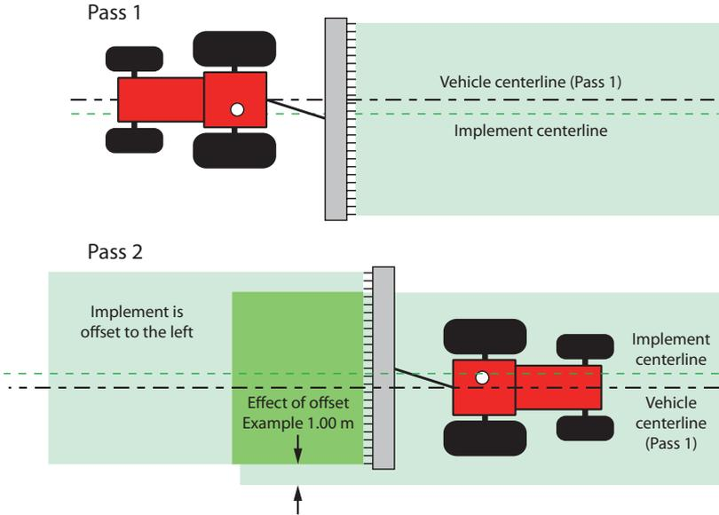
**Figure 2-6: Determining the effect of implement offset**
