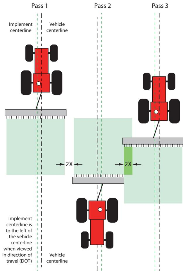
No implement offset entered. Skips and overlaps occur (2X). Direction of offset is Left when viewed in direction of travel.
