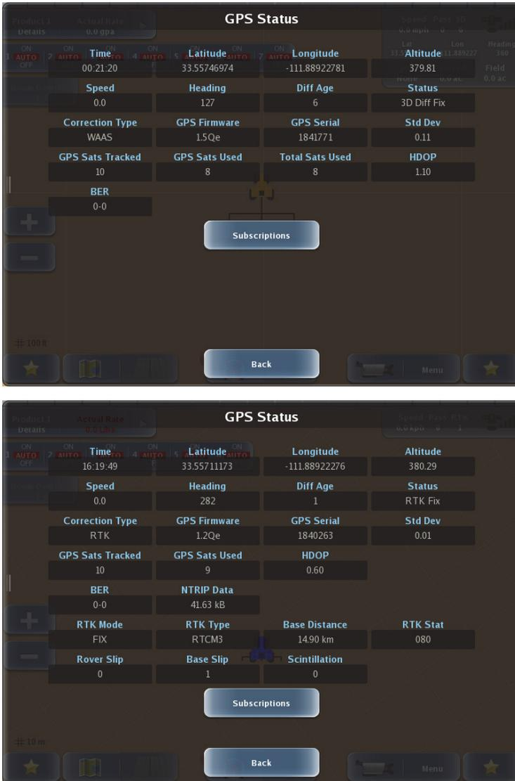
**Figure A-1: GPS Status screen (top - SBAS or OmniSTAR, bottom - RTK)**
