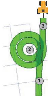
**Figure 2-9: Manual filter convergence driving sequence**
