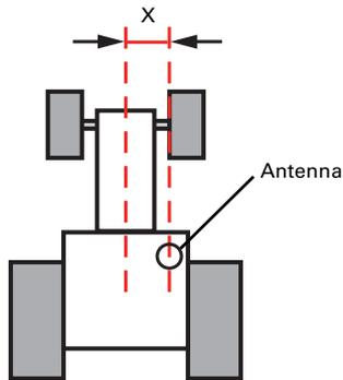
**Figure 2-2: Antenna offset (distance= X, direction = right)**
