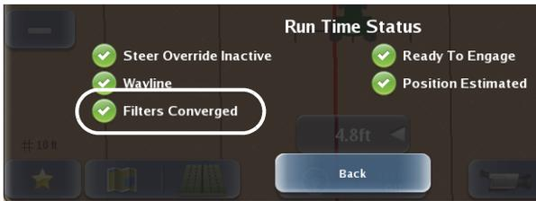
**Figure 2-8: Filters Converged checked on the eDriveX Status screen**
