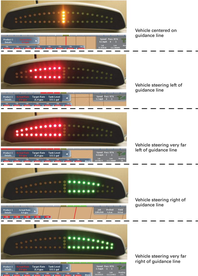
**Figure 8-2: Onscreen and external lightbar comparison**
