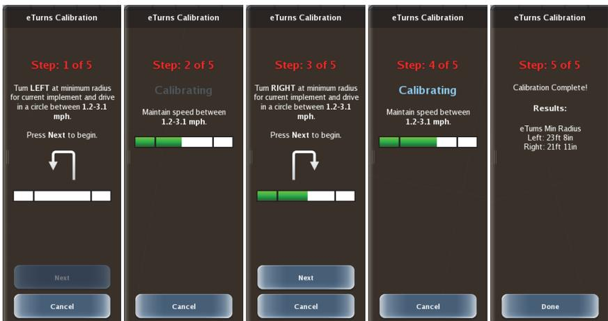
**Figure 6-4: eTurns calibration steps**
