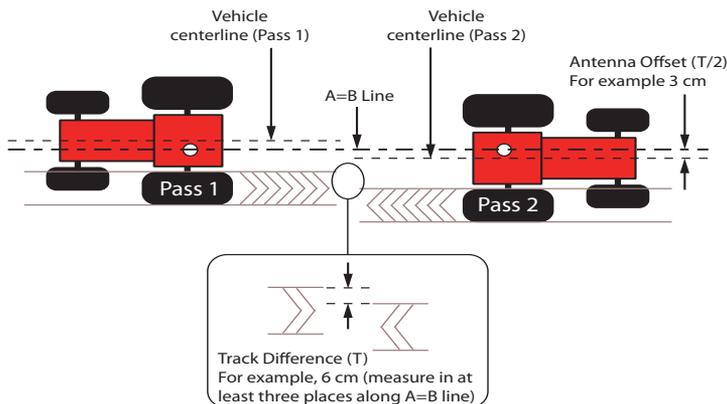
**Figure 2-3: Determining antenna offset (example  $6/2 = 3$  cm left)**
