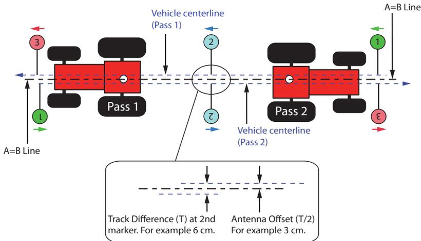
**Figure 2-4: Determining the antenna offset (example  $6/2 = 3$  cm left)**
