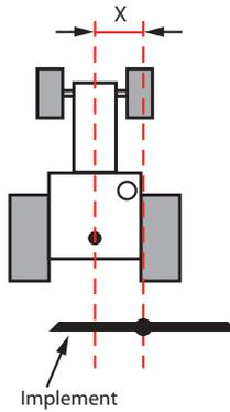
**Figure 2-5: Implement offset (distance= X, direction = right)**
