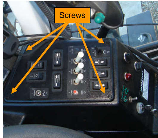
Fig. 1: Boom switch control panel
