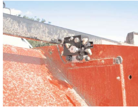
Figure 2c. Mounted automated steering block.
