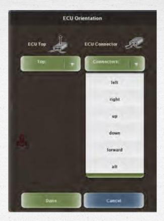
If ECU orientation is incorrect calibration will fail. NOTE: TOP is the side with the cooling fins.
