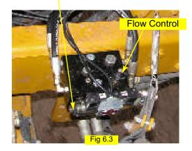
Note: To activate the manual overrides, a tool such as a small screw driver or allen wrench must be inserted into the end of the coil to depress the override button.
