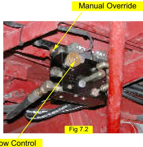
**Note:** To activate the manual overrides, a tool such as a small screw driver or allen wrench must be inserted into the end of the coil to depress the override button.
