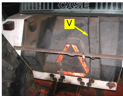
Figure 8b. Routed valve cable in cab.
