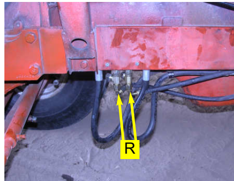
Figure 7b. Steering hoses connected to counter-balance valve..
