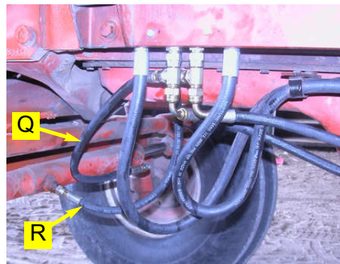
Figure 7c. Hoses connected between counter-balance valve and steering cylinder
