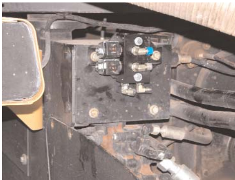
Figure 2c. Installed Automated Steering Block.
