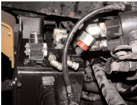
Figure 2c. Installed Automated Steering Block.
