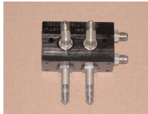
Figure 1c. Valve coils removed
